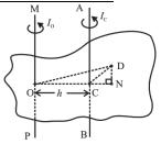
C be the center of mass M Object mass Axis of rotation MOP is parallel to axis ACB which is passing through center of mass and perpendicular to the plane. h is the distance between the
